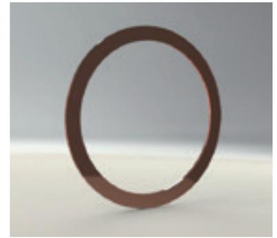
Oxygen free high conductivity (OFHC) copper is a suitable sealing material for bakeable UHV systems because of its good conformity with the thermal expansion coefficient of stainless steel as well as its essentially lower hardness (approx. 85 Brinell)
